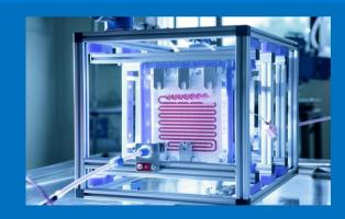
CPI: Corning Advanced Flow Reactor for Continuous Reactions
